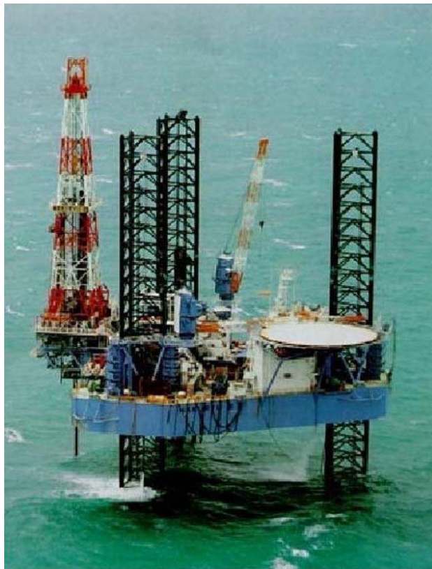
Figure 1: Jack-Up Drilling Rig with Triangular Shape and 3 Legs (JDC Hakuryu 8) (Reproduced Courtesy of Japan Drilling Co.)
