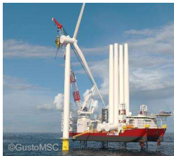
Charybdis WTIV First Jones Act Wind Turbine Installation Vessel 12MW+, 2,200-T Crane ABS Class Selected
