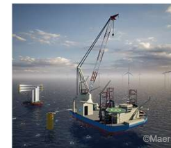
Maersk WTIV and Feeder Concept – Maersk WTIV combined with Eco tugs and barges ABS Class Selected
